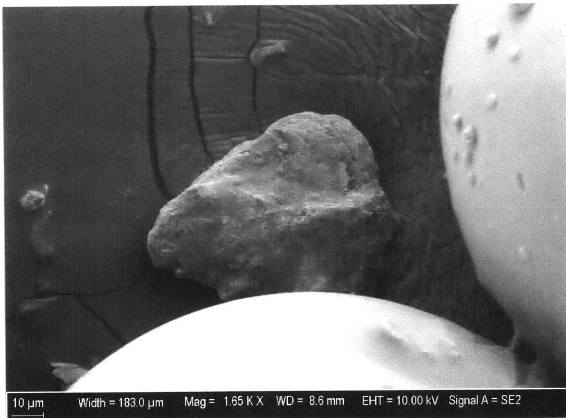
Figure 3-19 A typical organo-silicate particle from the anoxic Shewanella samples. Mineralization appears generally amorphous with some small lumps on the exterior. Some similar particles had slightly more structure, but typically clear crystal faces were not present. According to the Expert ID and Quant functions on the SEM, EDS scans of the center of this image revealed abundant C, O, Si, up to 10% Fe, and lower levels of Al, and Mg.
