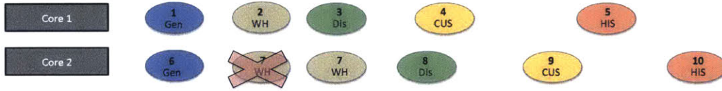
Figure 4-2: Execution sequence of 2 payment txns in a 2-core system.
