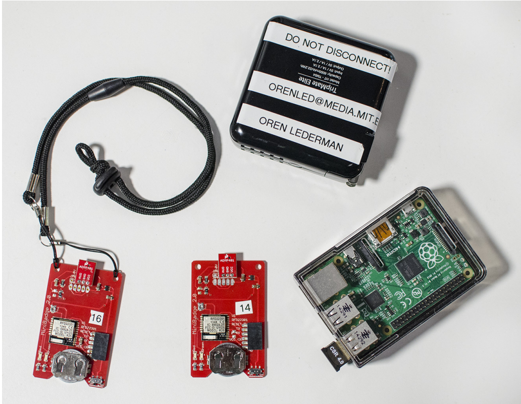
Figure 3-1: A simple deployment that includes two badges, a base-station, and a portable Wi-Fi access point
