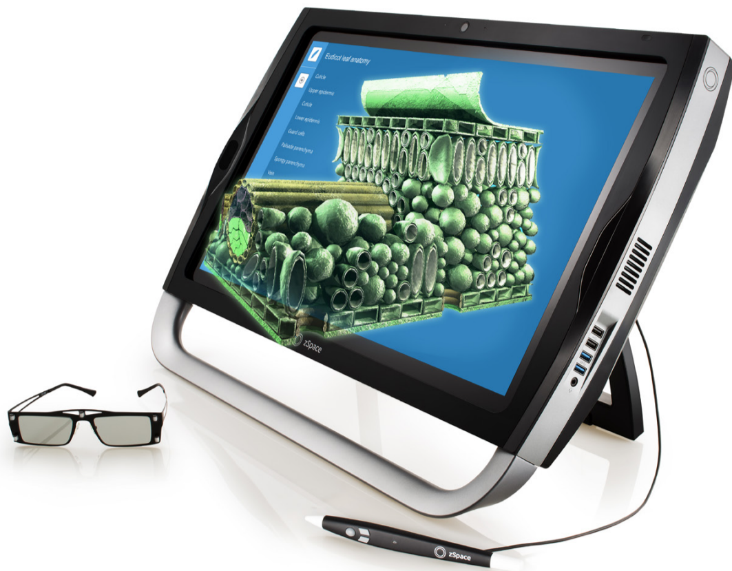
FIG 5.11.1 - The ZSpace display, with glasses and a 3D stylus used for interaction in ZSpace application demos (not used in HoloSuite).
