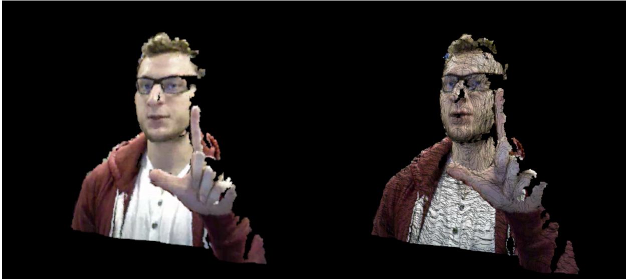
FIG 5.7.1 - This scene is taken of a user facing the depth camera, and the resulting 3D data is rotated to visualize the side angle of the face. On the left is the simple point cloud representation of a segmented user, the right image shows the scene from the same angle using fast mesh implementation from Point Cloud Library. Notice that the edges and holes on the mesh are much more difficult to tolerate visually. In the point cloud we can cover and smooth these simply by changing the size of the points.
