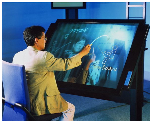
FIG 3.3.2 - The ClearBoard seamless layout, showing two remote users collaborating on a single display space.
