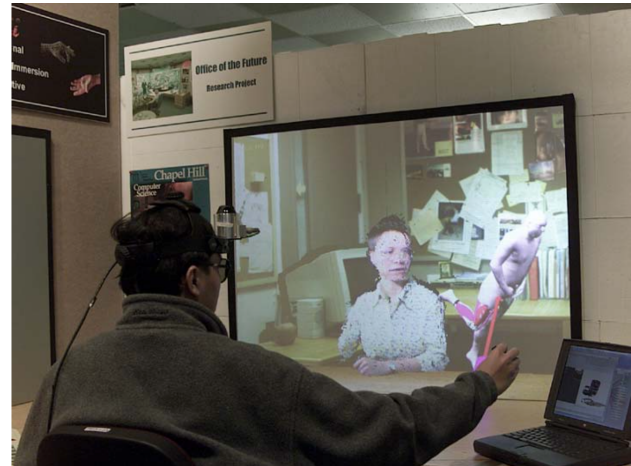
FIG 3.2.1 - End-to-end 3D telepresence in 1998 showing two users manipulating a 3d model with a pointing device [10].
