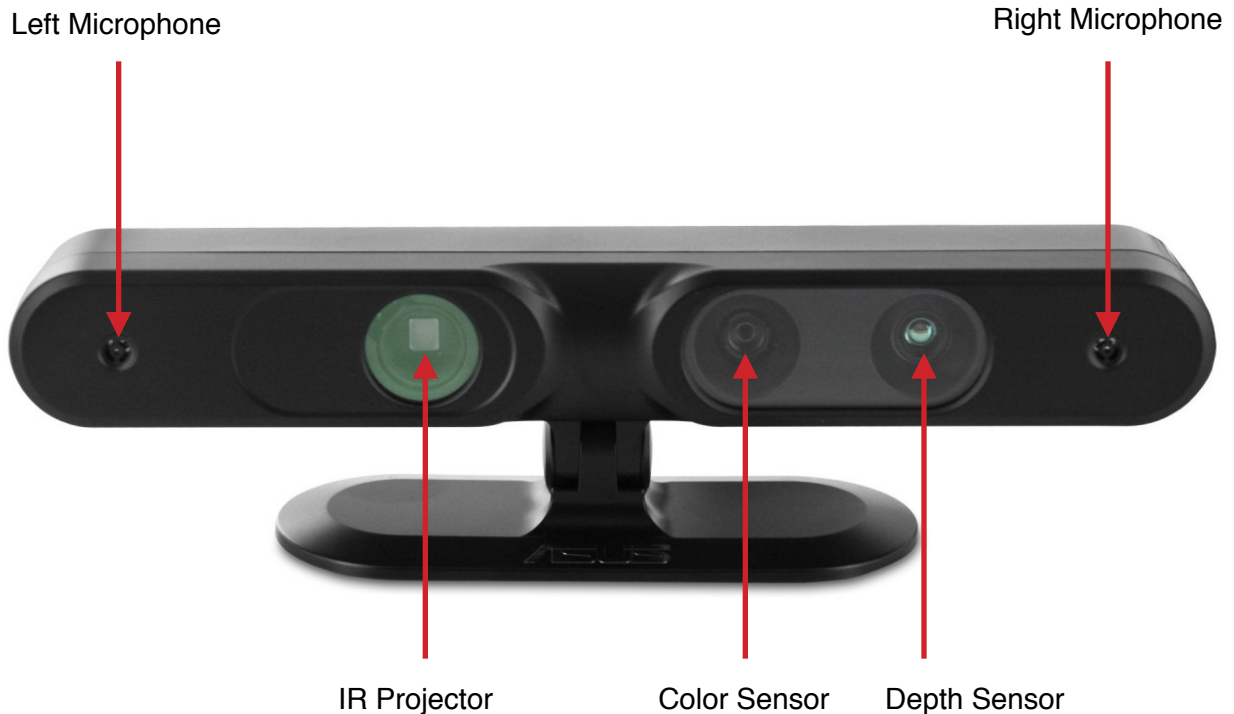
FIG 5.2 - ASUS XTION Pro Live is a commodity depth-sensing camera with stereo microphones, a structured-light depth sensor operating in IR spectrum with an RGB sensor for color image capture. The unit is self-powered via USB 2.0 port, giving data similar to the Microsoft Kinect with a smaller footprint and no need for external power supply.
