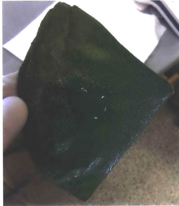
Figure 4-4: Photograph of a lotus leaf after spraying opposite polyelectrolytes (Chitosan/ Alginate).
