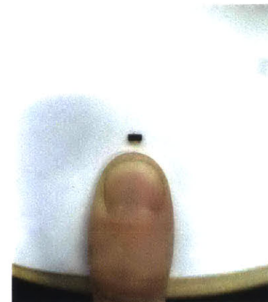
Figure 3.1.3 A single outline transistor in a SOT-23 package with my thumb for scale. It is important to note that the actual transistor is at the nano-scale. What you see here is the outer plastic casing.
