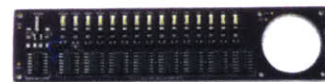
Figure 4.2.2.6 Proof of concept to visualize the reduction of 32,768Hz into a 1Hz signal before it goes to the motor. Built with CD4013 and CD40106 ICs.
