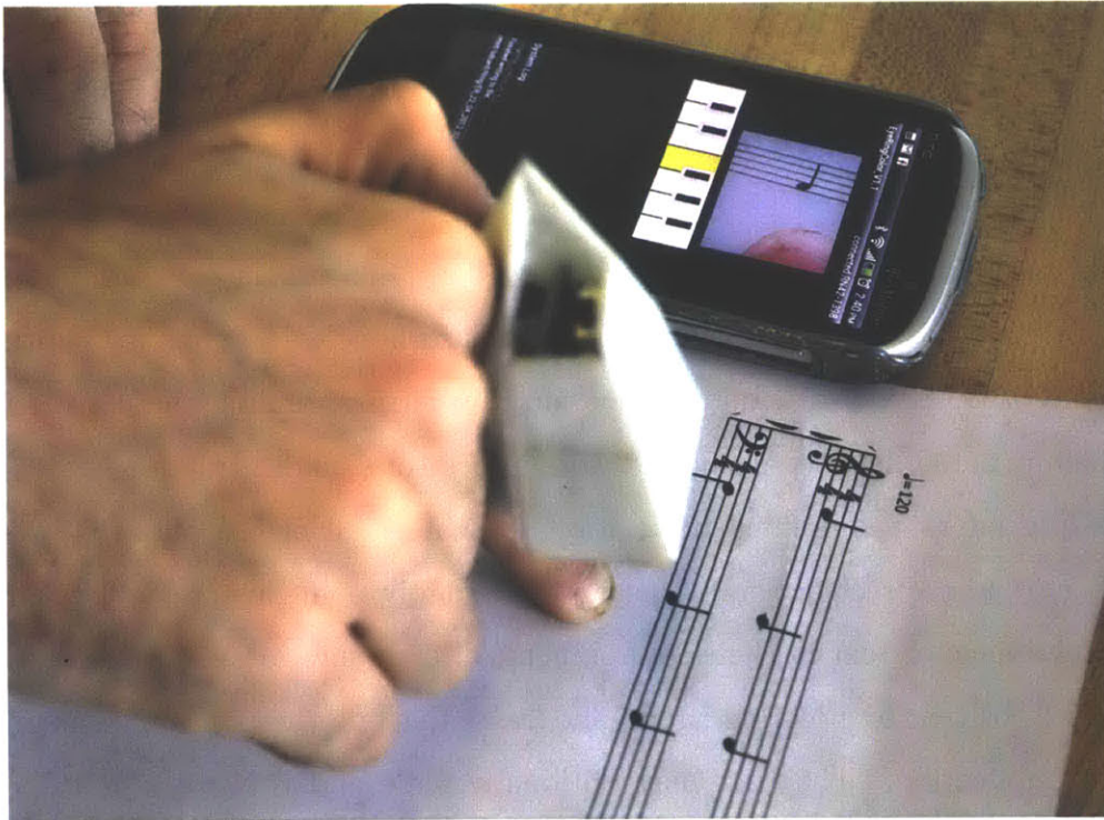
Figure 3-7: The sheet music reading system. A user points his finger at a note and hears it played out and displayed on screen
