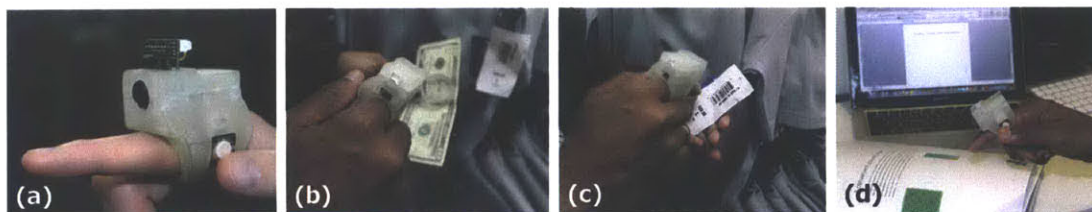
Figure 3-1: EyeRing: A finger-worn input device. (a) EyeRing prototype. (b) CurrencyDetector application. (c) TagDetector application. (d) Interaction with printed media.
