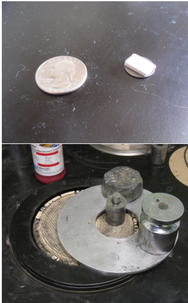
Figure 5-1: [Top] Sample mounted on AFM disc. [Bottom] Polishing instrumentation with jig and holder.
