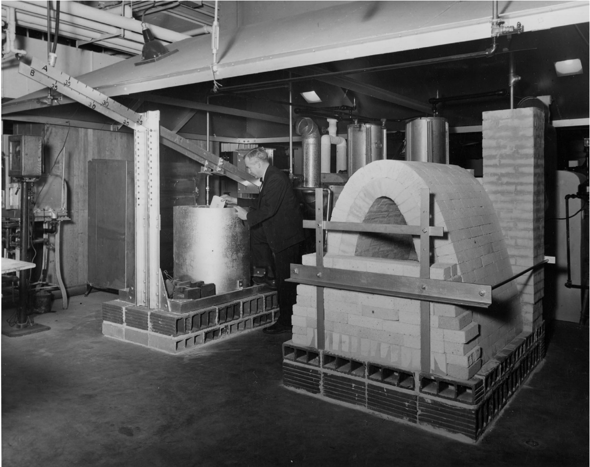
Figure 9 Wilkes preparing refractory bricks to be tested under load at temperatures up to 1540^{\circ}\text{C} (c. 1939). At right is a gas-fired kiln, the arch of which is a perfect catenary.
