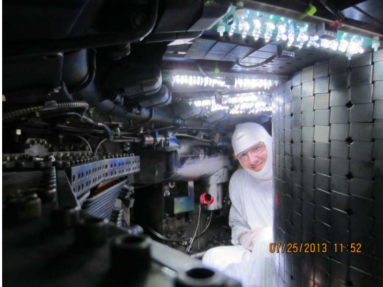
The author inside the tokamak working on the MSE diagnostic. The red glow is the LEDs from the MSE's ISC system.
