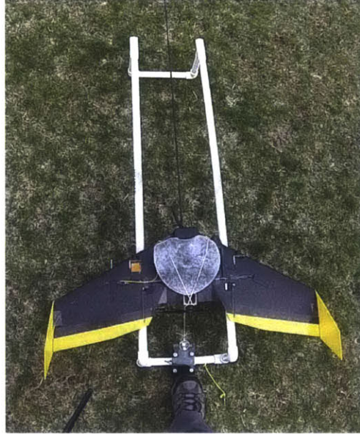
Figure 2-4: Aircraft hardware in the field. We use a small catapult for consistent launches near obstacles.
