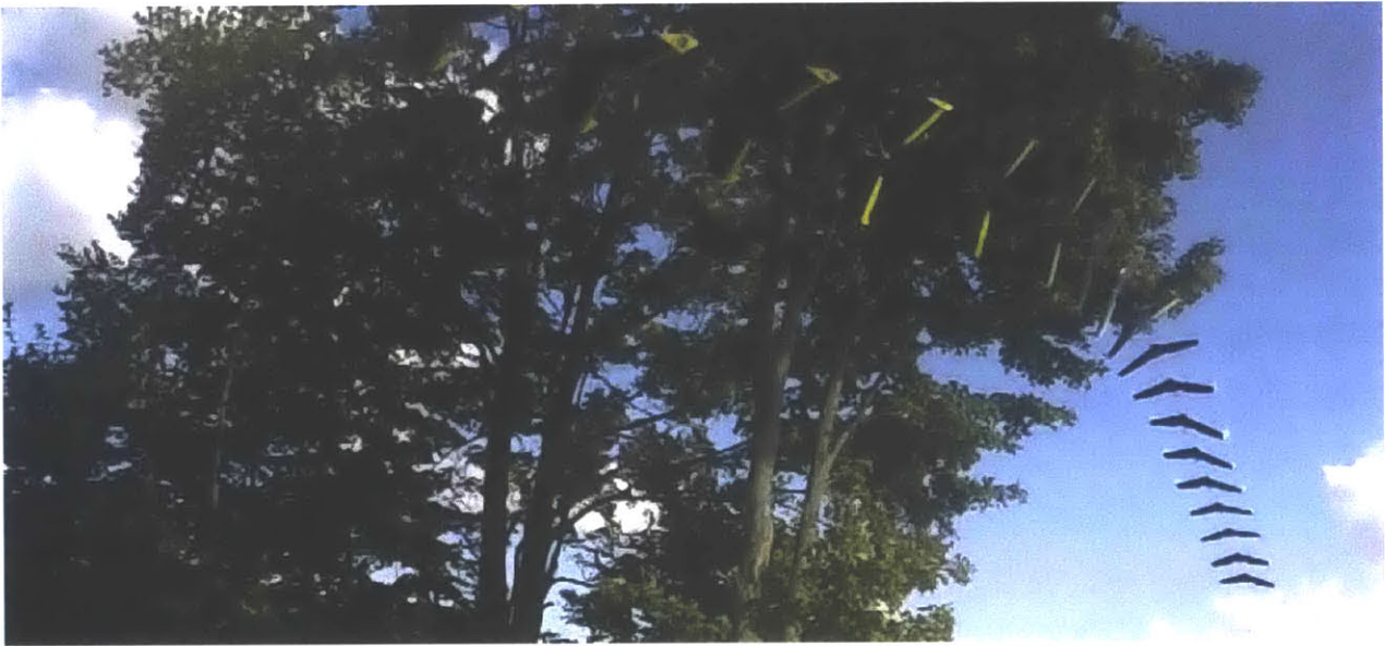
Figure 4-11: Aircraft avoiding obstacles as viewed from a camera mounted on the tree seen in the left of the images in Figure 4-10. Each snapshot is 0.083 seconds apart and the total sequence spans 1.4 seconds.
