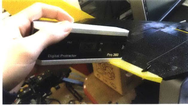
Figure 3-3: Measuring servo deflection for a given input.
