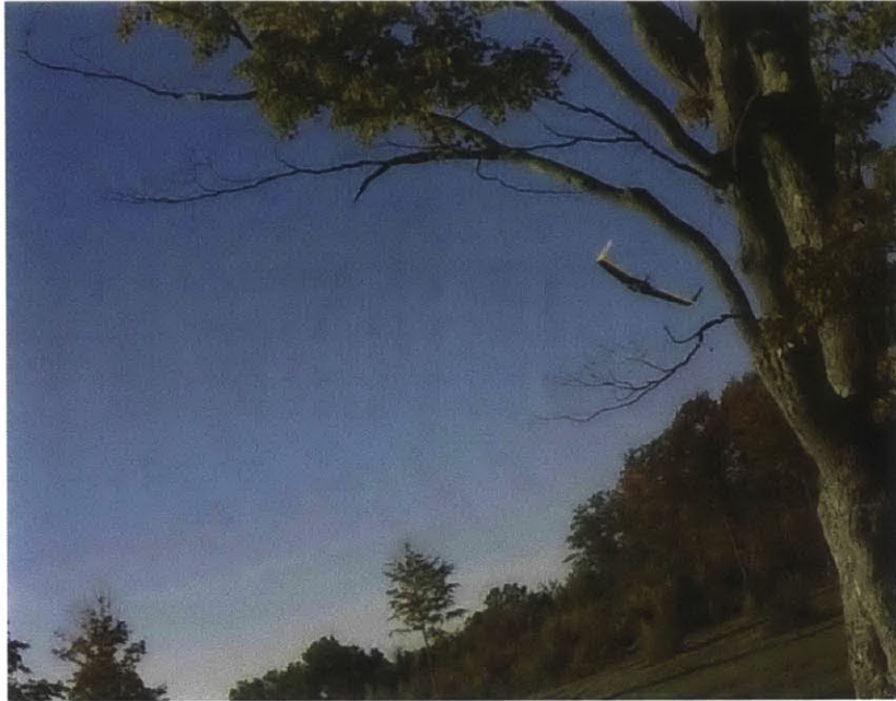
Figure 4-8: Chase camera view of the autonomous aircraft avoiding a tree.
