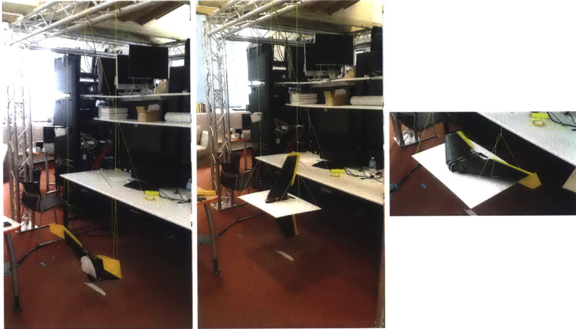
Figure 3-6: Measuring the moment of inertia with a bifilar pendulum (roll, pitch, and yaw axes respectively). The technique involves measuring the period of oscillations about the axis in question.
