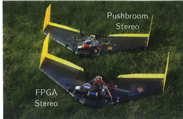
Figure 2-12: Experimental aircraft platforms holding the pushbroom stereo system (back) and the FGPA stereo system (front). Cameras are mounted on the front of the wings at the same baseline (14 inches) on both airframes. Covers over the electronics were removed for this photograph.
