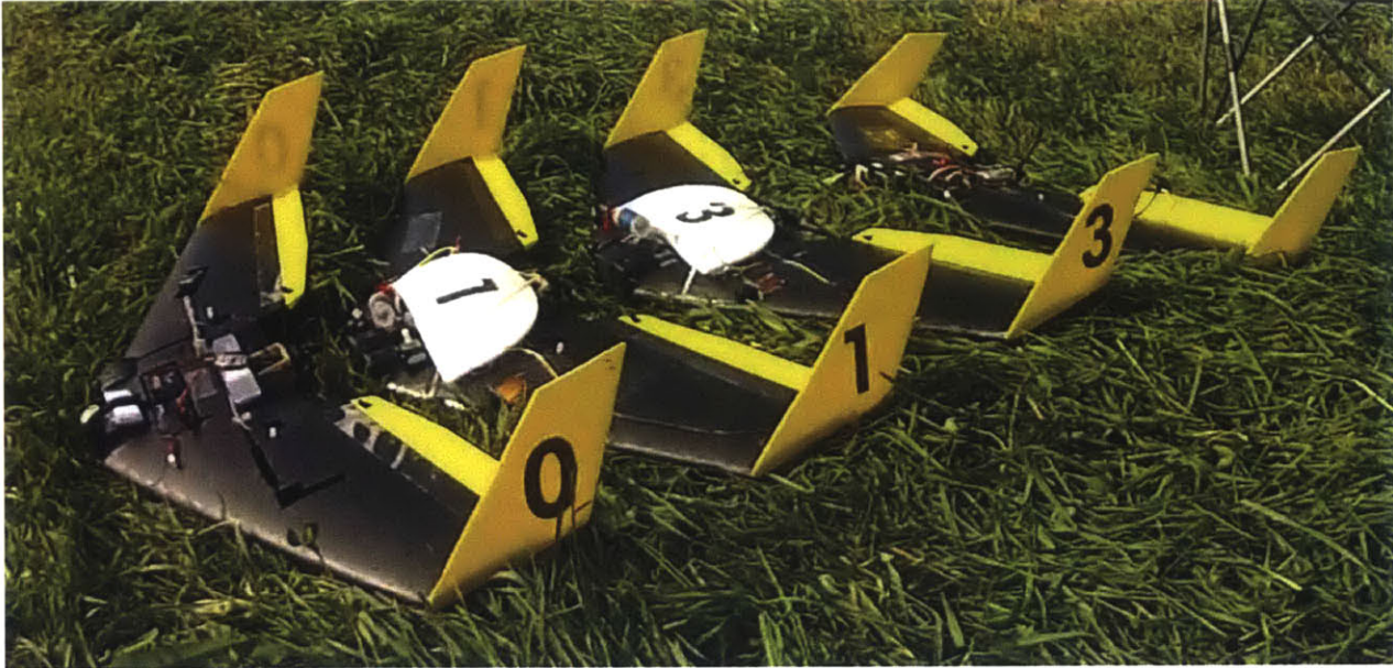
Figure 4-2: Set of flight aircraft. Numbers 1 and 3 are equipped for autonomous flight.
