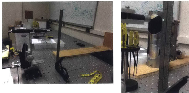
Figure A-2: The setup for the alignment of the laser pointer will be used to align in-vessel mirrors in the canister.
