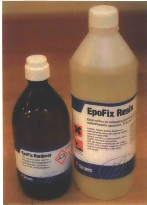
Figure B. 10: Struers EpoFix epoxy system used to mount TRISO particles.
