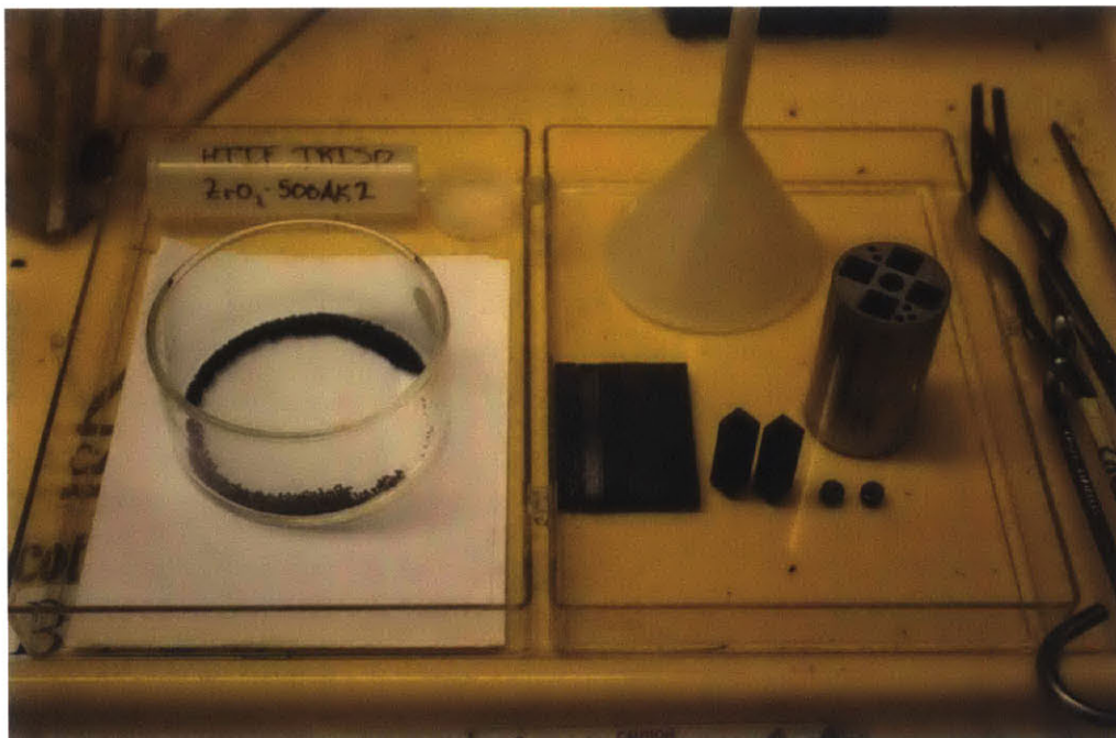
Figure A. 9: At left, irradiated surrogate TRISO particles from the HTIF sample capsule. At right, HTIF sample capsule and graphite specimens from that capsule.
