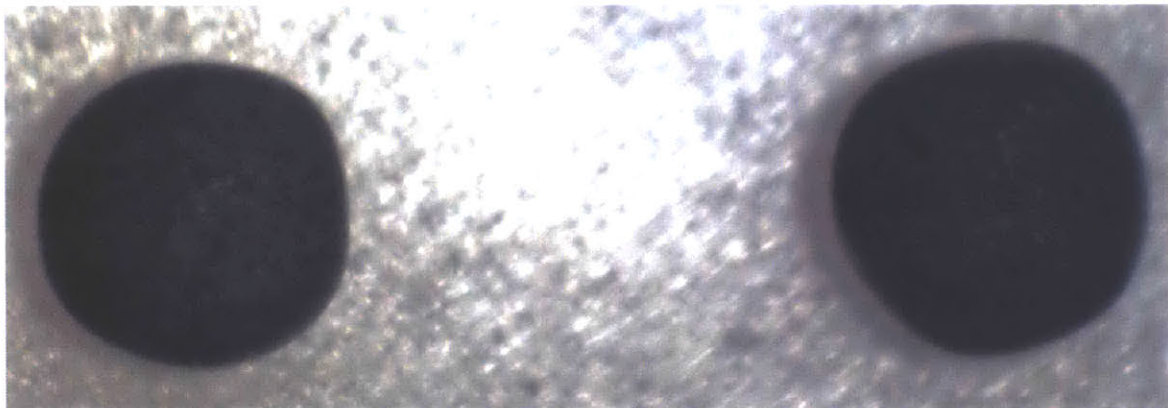
Figure 4.14: Particles from UW test in flibe after additional freezing and thawing cycles in flibe at MIT.
