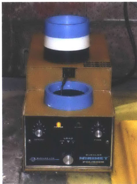
Figure A. 10: Buehler MiniMet in fume hood certified for work with radioactive samples.
