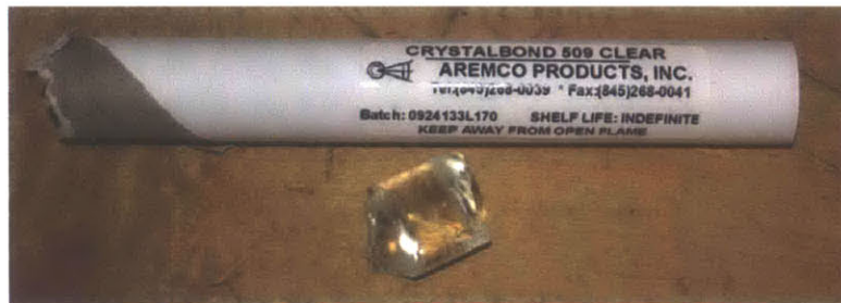
Figure B. 8: Crystal Bond 509 used to affix TRISO particles to bottom of mounting cup.
