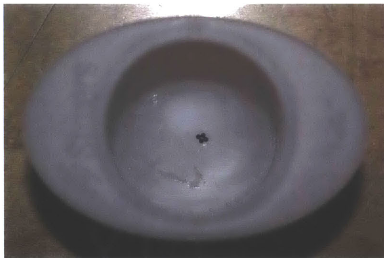
Figure B. 9: Four as-fabricated TRISO particles affixed to the bottom of a mounting cup with a thin film of Crystal Bond.
