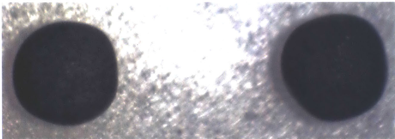
Figure A. 58: Particles from UW test in flibe after additional freezing and thawing cycles in flibe at MIT.
