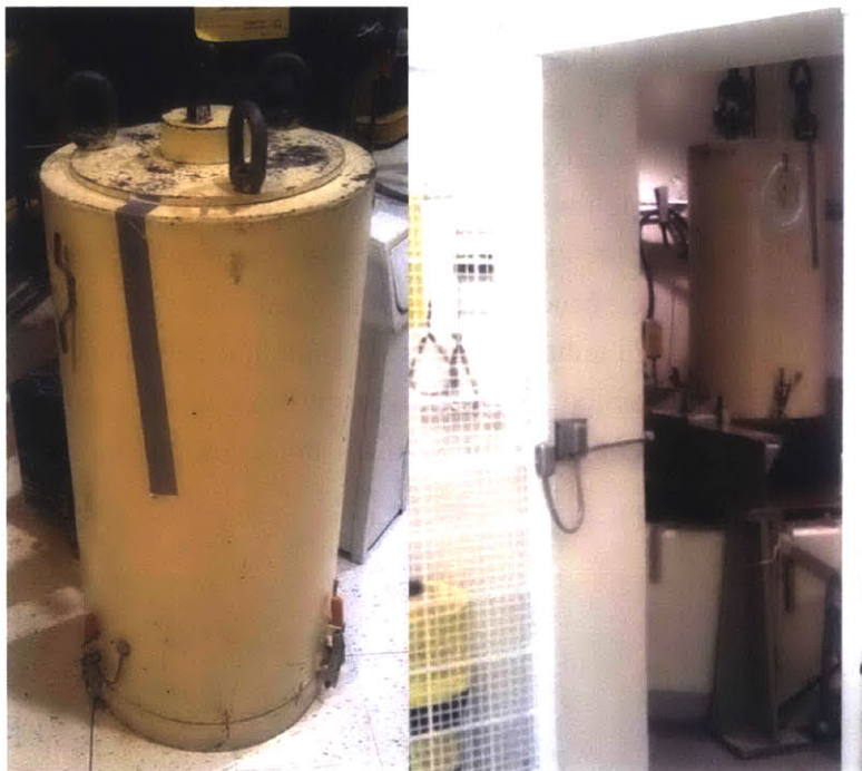
Figure A. 5: At Left, the cask used to transfer the HTI. At Right, the cask being raised from the spent fuel pool bridge.
