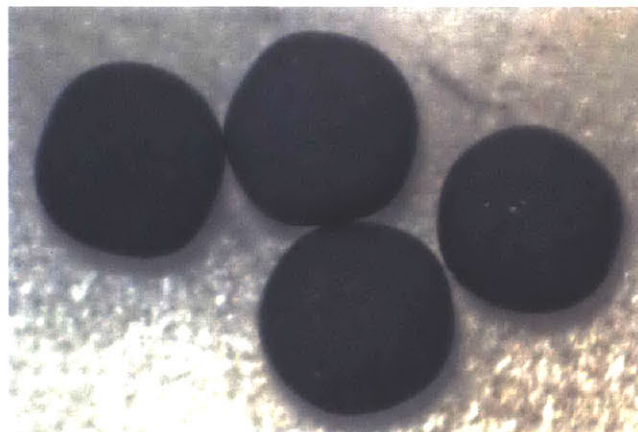
Figure A. 50: As-fabricated TRISO particles from batch ZrO 2 -500-AK2.
