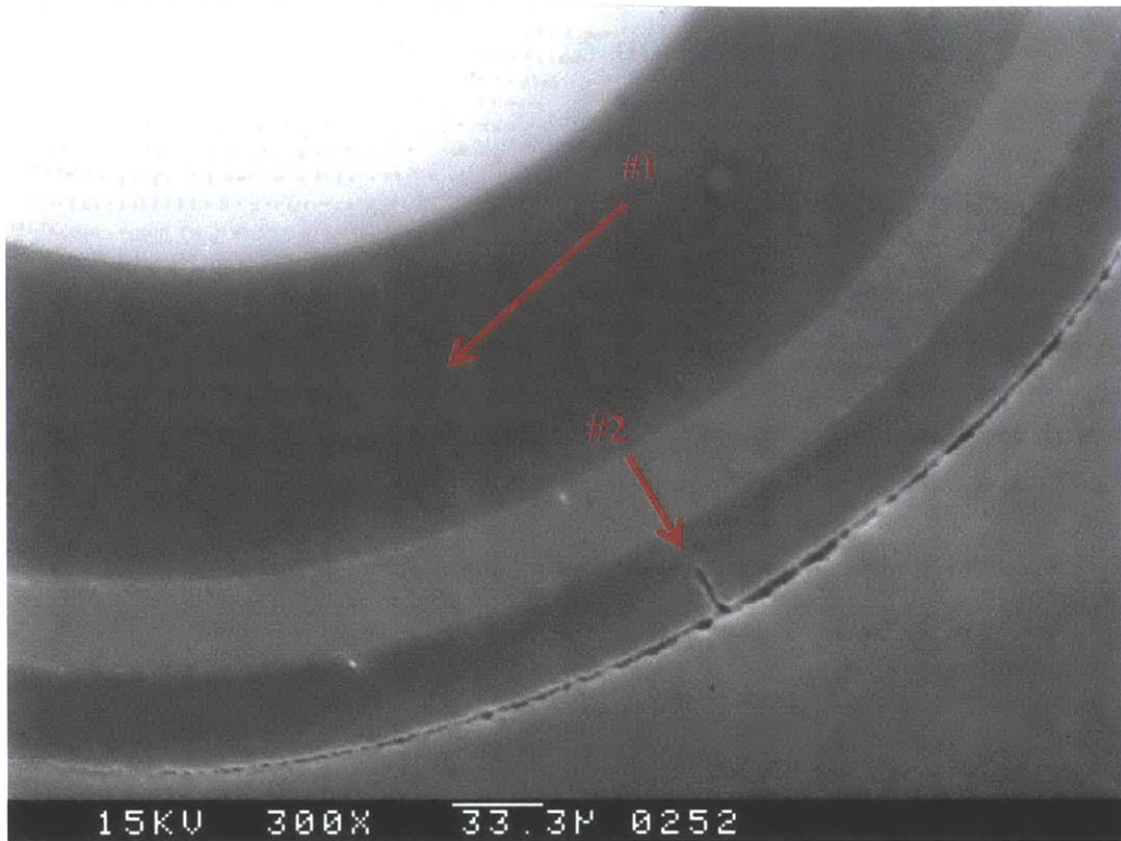
Figure C. 40: 300x SEM micrograph of mount I2 particle 13. Arrow #1 indicates buffer and IPyC crack. Arrow #2 shows OPyC crack and gap between epoxy and OPyC.
