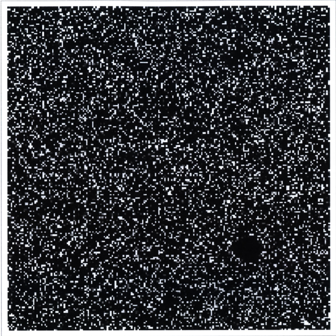
Figure 49. Results from a transmission simulation for a weapon enclosed in a 2 m x 2 m x 2 m container. Cargo was randomly populated with low- and medium-Z material for every cc surrounding the weapon. A dark spot in the lower right of the graphic shows the presence of the weapon.
