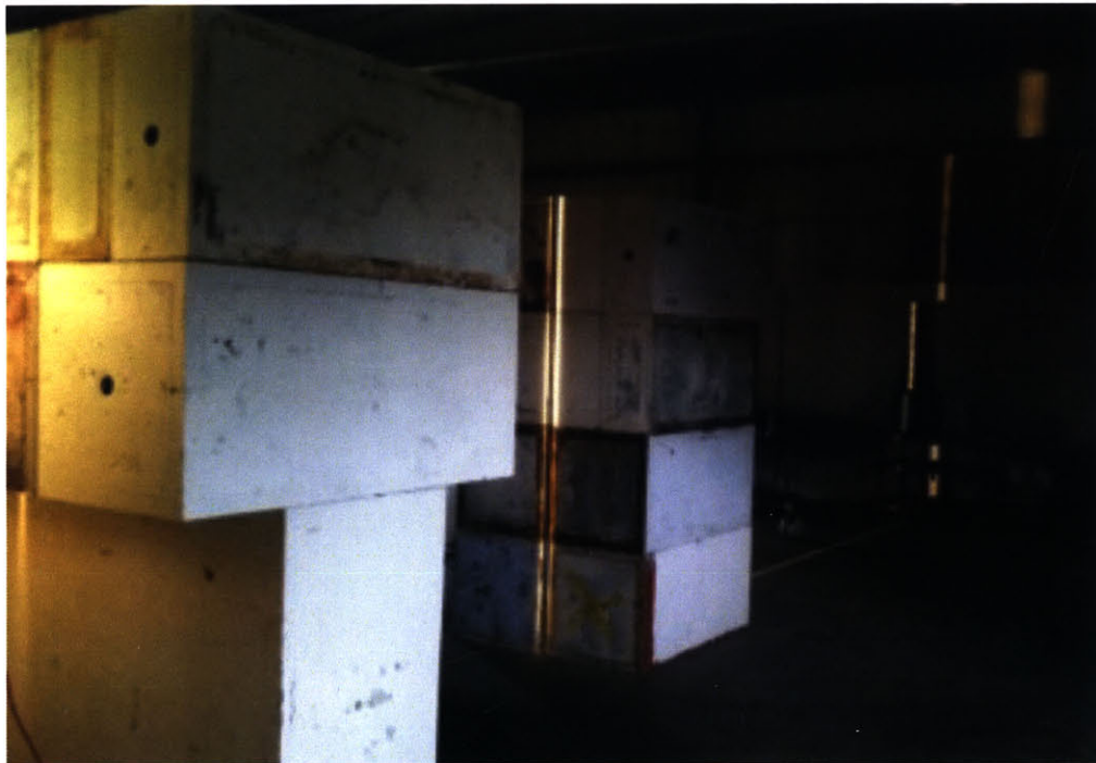
Figure 21. Double density concrete collimators. A flood light was used to shine light through the collimation channels to verify the detector array was correctly positioned in the beam line. Cargo to be scanned was placed in the beam line between the two sets of concrete collimators.
