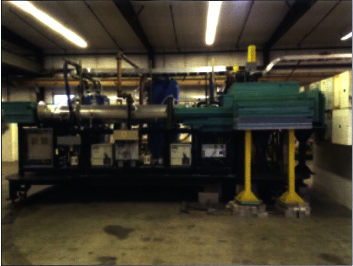
Figure 56. DL-3 accelerator with shielding in place. Note the HDPE to the back (left) of the accelerator to shield for neutrons traveling back through the vacuum.
