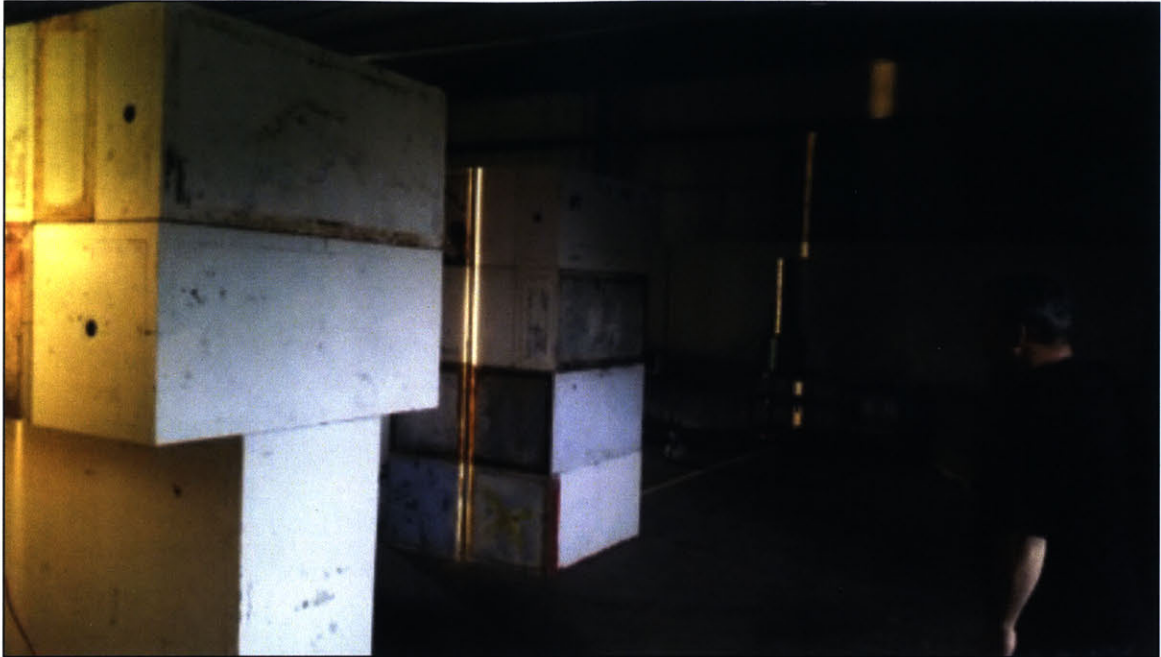
Figure 60. Using light to confirm daily alignment of the NaI(Tl) array with the beam line. Note the first and second sets of double density concrete collimators.
