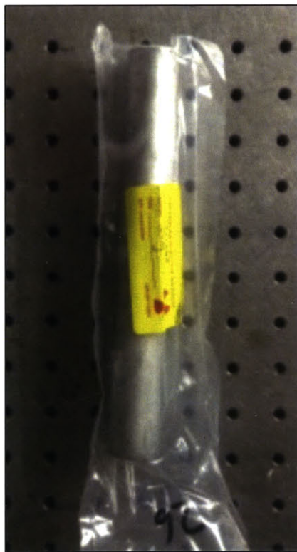
Figure 63. A 1.1" U rod used in the experiments. The rod had an aluminum housing and a U diameter of 0.93".
