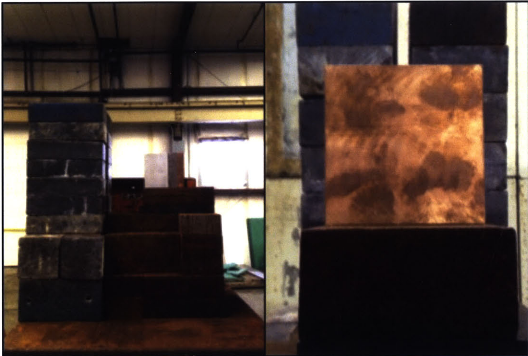
Figure 22. Pb collimator immediately after cargo. The Pb collimator was placed immediately after the interrogation cargo to limit the amount of scattered radiation entering into the beam line. Keeping a gap between the interrogated cargo and Pb collimator limited the acceptance angle for scattered radiation into the beam line.
