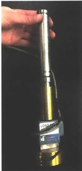
Figure 3-19: The piston, attached to a spacer, then the load cell, and finally the alignment cap that fits with and aligns the top endcap. The alignment cap seen here has the ability to connect to the piston to enable suction; however, this was not used in this research. The standard top cap used in this research did not rigidly connect to the piston
