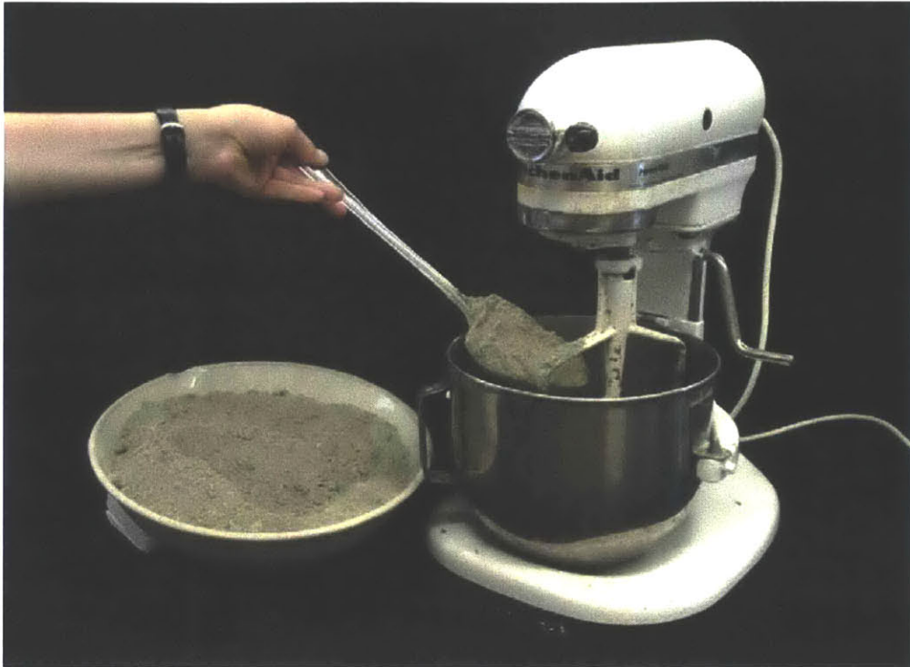
Figure 3-12: This is the second step of resedimentation, where clay powder is mixed with saline water until thoroughly homogenized and no lumps are present
