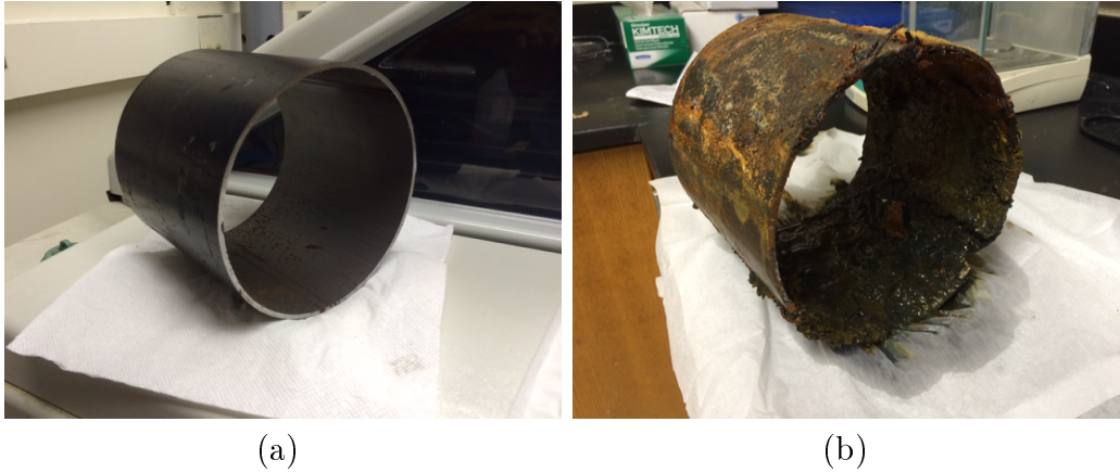
Figure 5-24: (a) An intact 6" Schedule 10 pipe, (b) a corroded 6" Schedule 10 pipe even cut surface, the 2 day corroded pipe with mild corrosion around the rim, and the 5 day corroded pipe with some parts darker than others and thinner as well due to the mass loss from corrosion.
