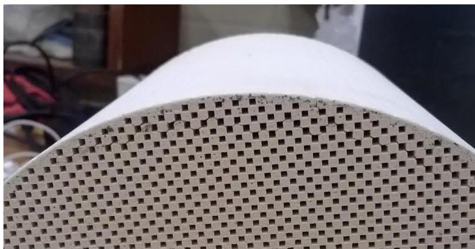
Figure 4.13: Cracked Exit Channels on Ca Filter 1
