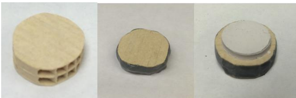
Figure 3.4: The Stages of Wafer Sample Preparation and Loading
