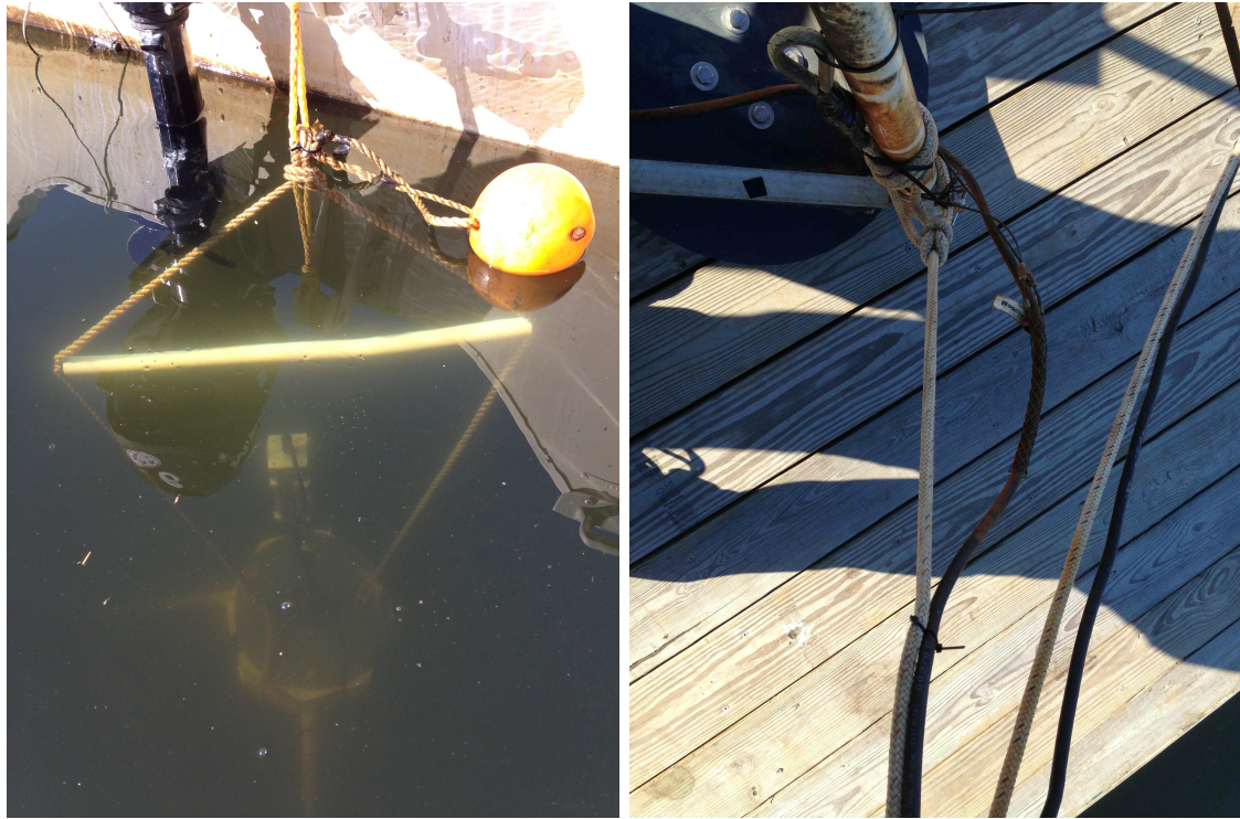
Figure 2-9: Left: photograph of the lander suspended by its top harness from the back of a boat, before being towed slowly underwater to its deployment location. Right: photograph of a base corner of the tripod before deployment, showing both rope and data cable strain-relief loops attached to a PVC leg of the tripod. These were critical in preventing damage to the sonar when the tripod was accidentally lifted by the data cable when an anchor snagged it. Beneath those is visible the quick-release pin holding the PVC leg into the speed rail aluminum corner fitting, one edge of the aluminum triangular base, and a round PVC pad to prevent significant settling into the mud.
