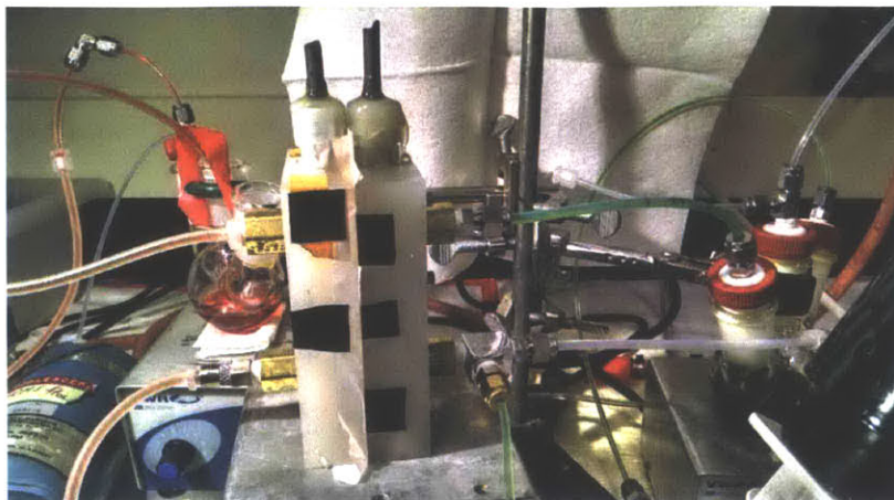
Figure 6.4 Experimental set up for CO 2 capture using flow-through electrodes. Liquid paths are highlighted using solutions of red and green food dye.
