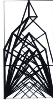
Figure 5-16: Trans. Tower Red. Optimal for a \frac{1}{2} H-W ratio and 6 \times 6 density
