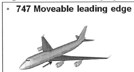
Figure 1-8: 747 Moveable leading edge [23]
