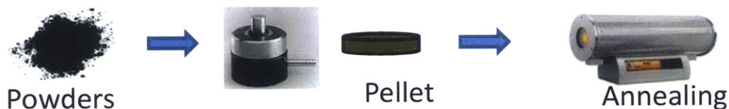
Figure 21. Schematic of solid-state synthesis for lithium transition metal oxides. This method has been used for most synthesis of lithium transition metal oxides rather than \text{LiNi}_{1/3}\text{Mn}_{1/3}\text{Co}_{1/3}\text{O}_2 . For solid-state synthesis, the starting materials are mixed in a stoichiometric ratio and grinded at least thirty minutes to get a homogeneous mixture. A pellet is done from this homogeneous mixture and annealed to high temperatures. Courtesy of Magali Gauthier and Thomas Carney.
