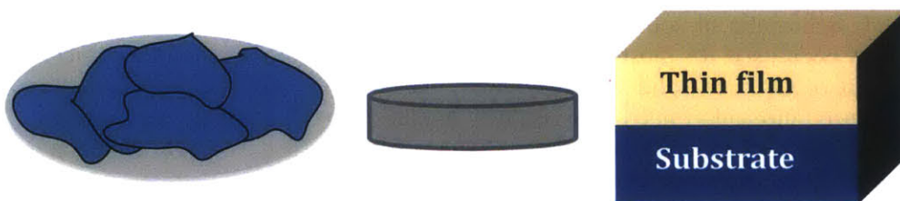
Figure 20. Model electrodes with 100% active material: Powder on aluminum discs (for XPS measurements), pellets (for XAS/XES measurements) and thin films, respectively. Courtesy of Magali Gauthier.
