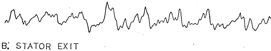
FIG. 15 HOT WIRE SIGNAL AT UNTREATED STATOR INLET AND DISCHARGE IM = .75 , STALL POINT
