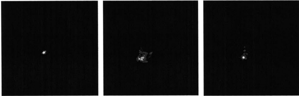
Figure 6-12: Closed loop mirror correction (left) before turning on the mirror (middle) after introducing aberrations (clear plastic sheeting) and (right) after 5 iterations of the algorithm.
