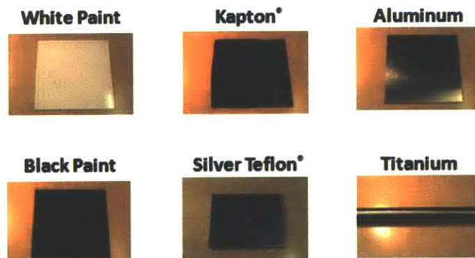
Figure 13: Pictures of “coupon” samples of spacecraft materials for Experiment A
