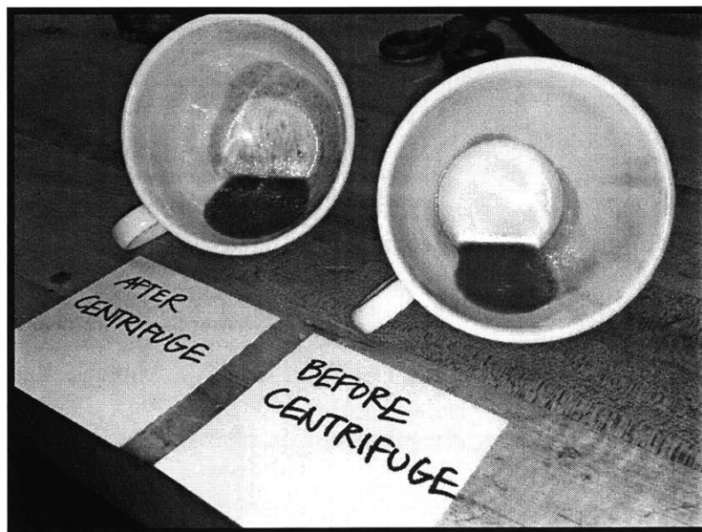
Figure 15: Comparing Pre/Post Centrifuge Avocado Mash Avocado mash before and after centrifuging. There are large oil drops present on the surface of the avocado mash that has been centrifuged, in comparison to the smaller oil drops on the sample.
