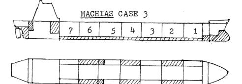
MACHIAS CASE 3: Double Bottom of depth 5.78 ft added to case 2 and the slop tank size is decreased.
