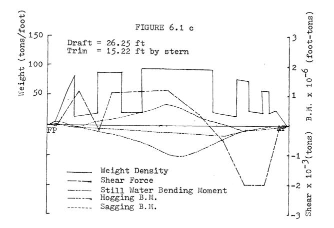
MACHIAS CASE 2: Longitudinal Bulkheads moved out 4.74 ft and slop tanks placed in Wkngs # 5. Ballast in Wings # 2, 4, 6 Slop # 5 Aft Peak Fore Peak Cargo in Centers # 1-7
