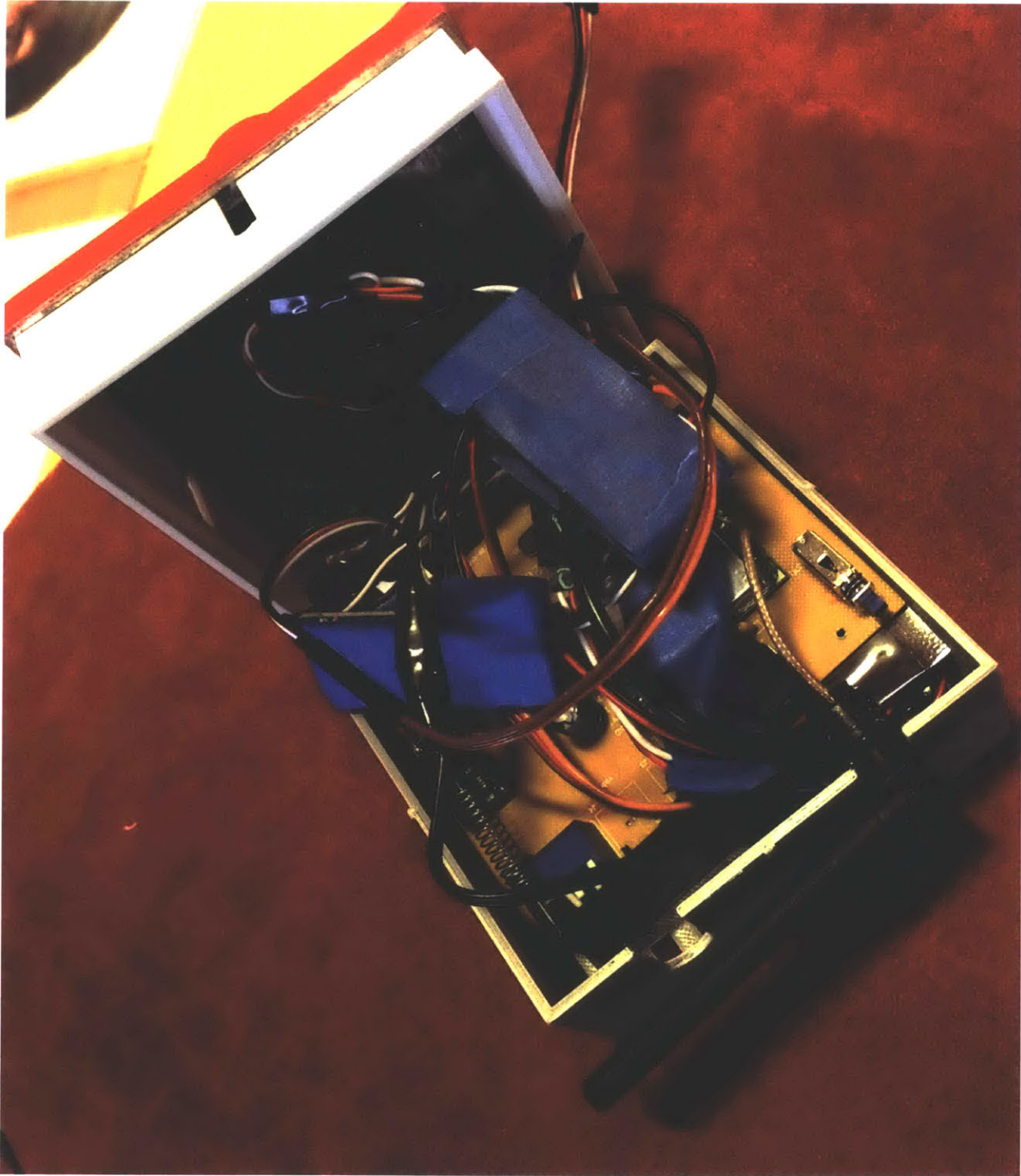
The housing contains battery pack, RF transceiver, amplifier and a microcontroller.
