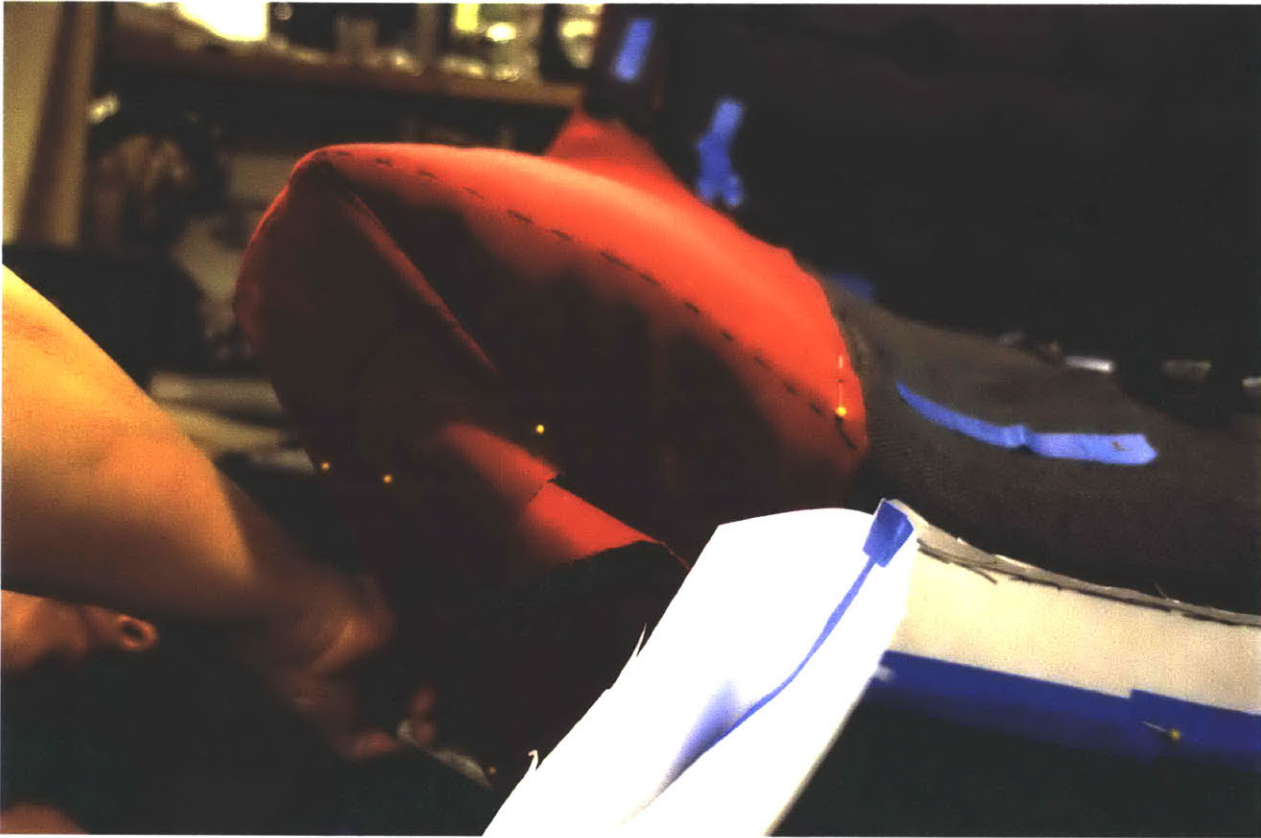
We used sponge to add extra padding to prototype the shape of the sofa.
