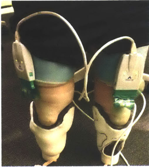
Figure 18: Tekscan F-Socket™ sensor inside a liner donned by a patient.
