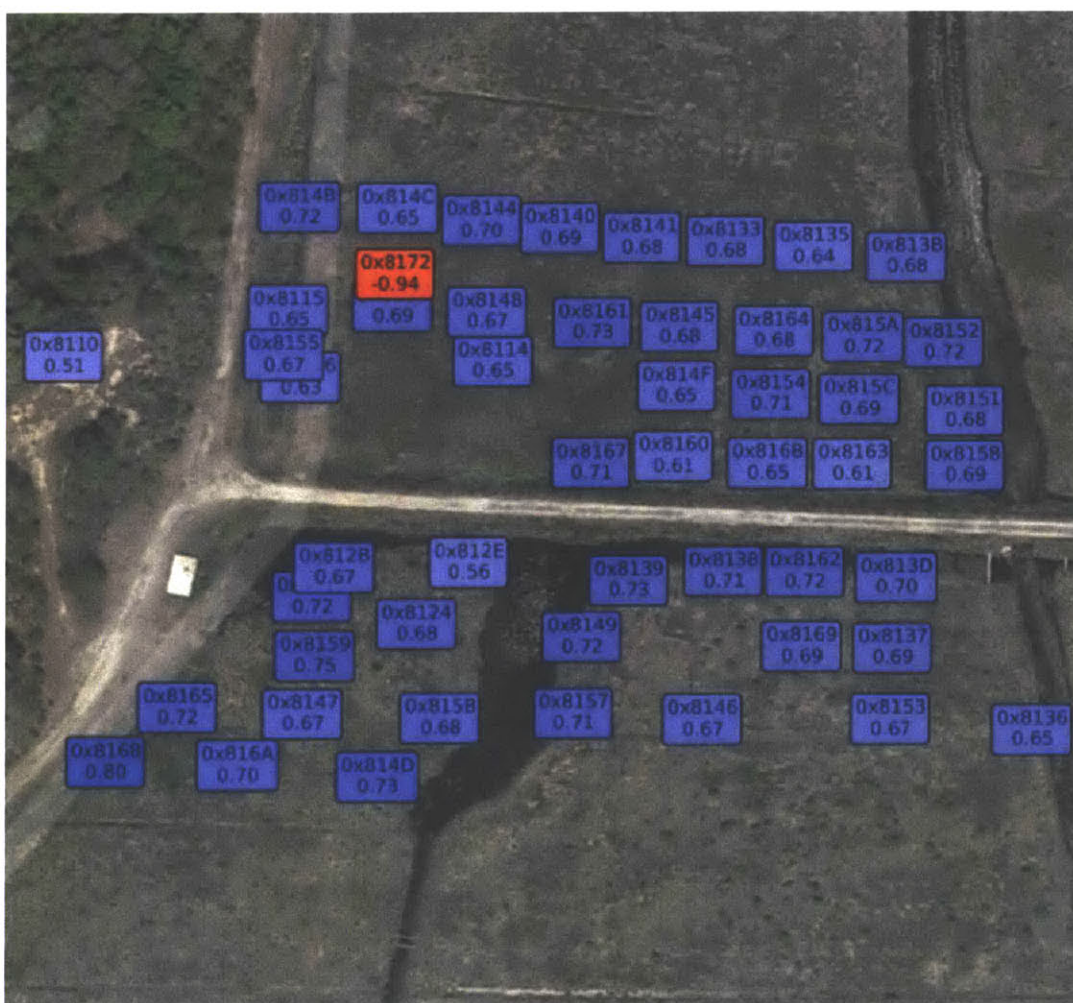
Figure 77. Hourly correlation between illumination and temperature hourly mean overlaid on aerial photo of sensor nodes. The sensor node in red produced a negative correlation because it was covered from external light. The internal light sensor was only exposed to an LED within the node that flashes when the node battery is discharging. Discharging occurs mainly at night, because the nodes are solar powered.
