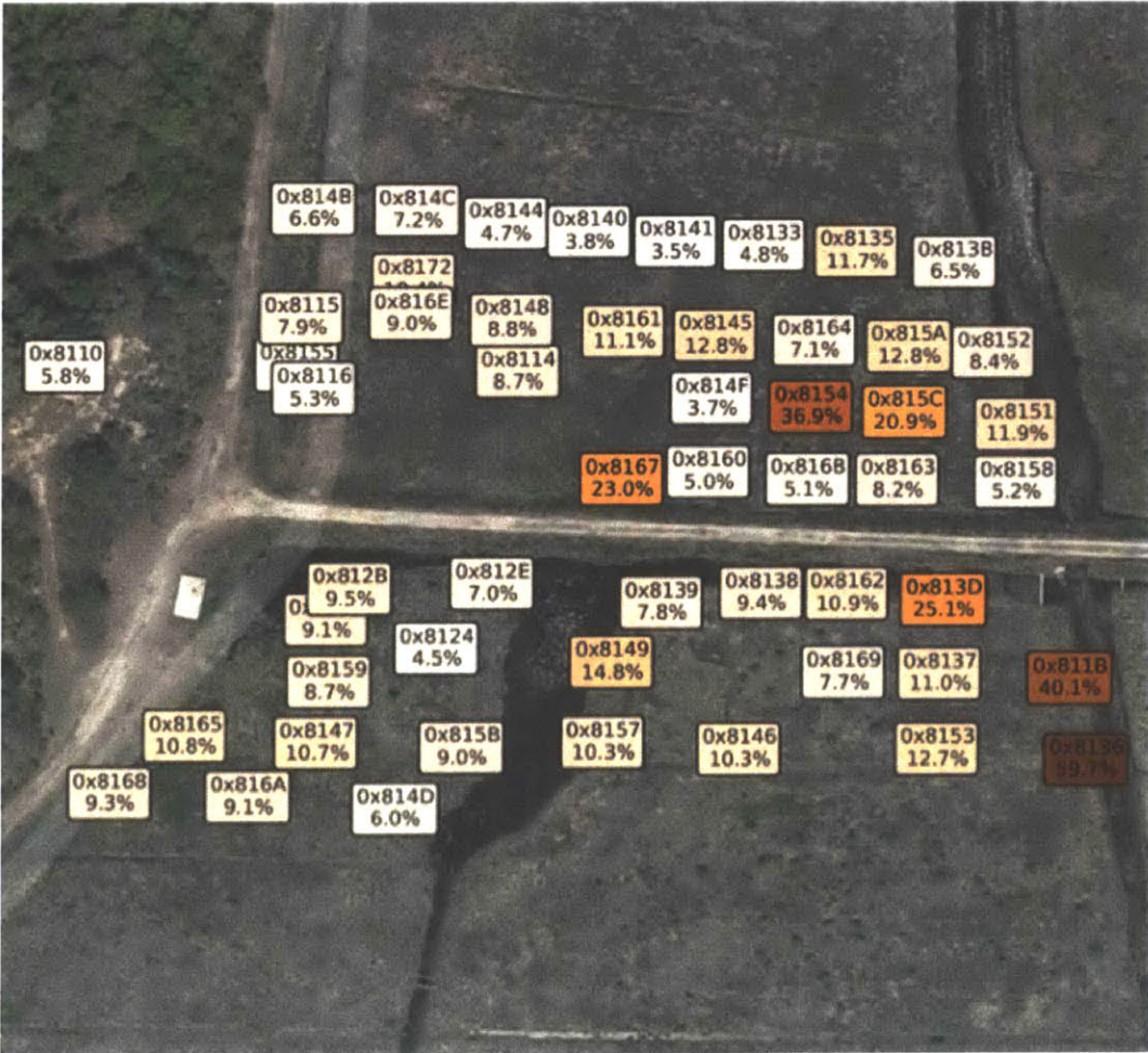
Figure 75. Packet loss rates overlaid on aerial view of sensor nodes. The two nodes on the bottom right that have the highest packet loss are located on a hill and therefore suffer from wireless connectivity problems
