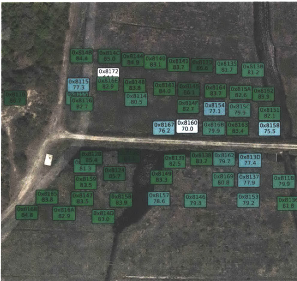
Figure 76. Average daily humidity overlaid on aerial view of sensor nodes
