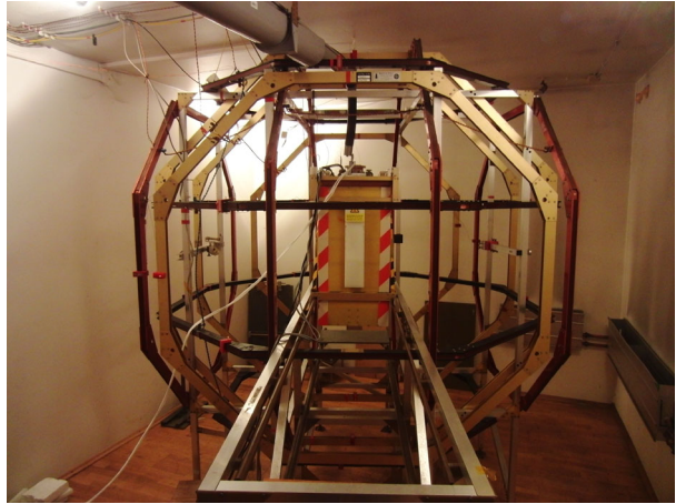
Fig. 3 The Magnetsrode calibration facility, a 2-m large Helmholtz coil system. A non-magnetic temperature chamber is placed in the center of the system
