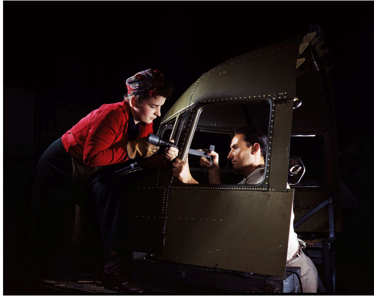
Figure 4. Ubiquitous solutions to construction problems. Alfred T. Palmer, Riveting team working on the cockpit shell of a C-47 heavy transport at North American Aviation, 1942, Library of Congress.
