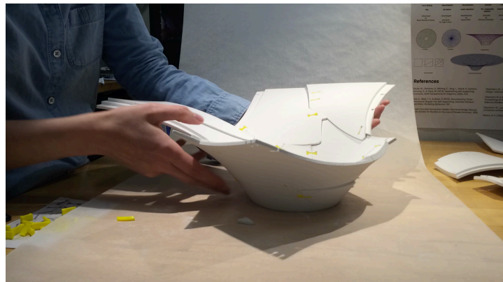
Figure 47. Need of external supports during assembly.
