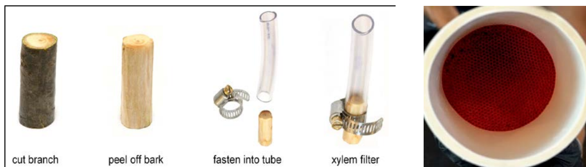
Fig 5: The measured flow rates 42 of about 0.05 ml per second using only \sim 1 \text{ cm}^2 filter area (left panel) correspond to a flow rate of >4 litres per day, sufficient to meet the drinking water requirements of one person. If a branch with a greater circumference was used to increase the filter area, will it affect the flow rate and quality of the filtered water? If xylem filter containing (narrow) tubes (left panel) were packed in a pipe with a larger diameter (right panel, illustration copied from laminar flow diagrams), can it help to scale and increase the volume of filtered water? Will the flow rate decrease? Will it affect water quality?
