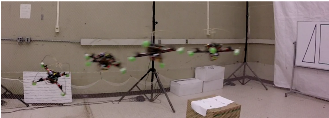
Figure 7-9: Raw Footage of Target Region Approach: Quadrotor flies aggressive angles; visual markers can be seen on the right.
