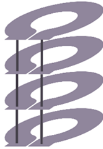
Figure 2-24: Winding structure for the resonant inductor. A detailed PCB layout and circuit board stackup for the windings is shown in Appendix D.
