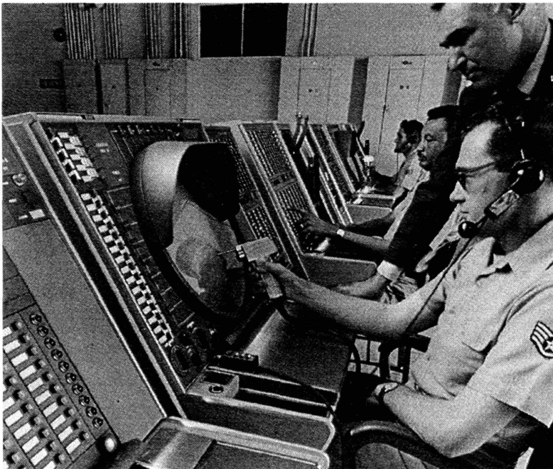
Figure 10-1: SAGE computerized air defense system. Note the role of the telephone network in the diagram above. Below, operators use “light guns” to designate targets on a computer-driven radar screen (Claude Baum, The System Builders: The Story of SDC (Santa Monica, California: System Development Corporation, 1981)).
