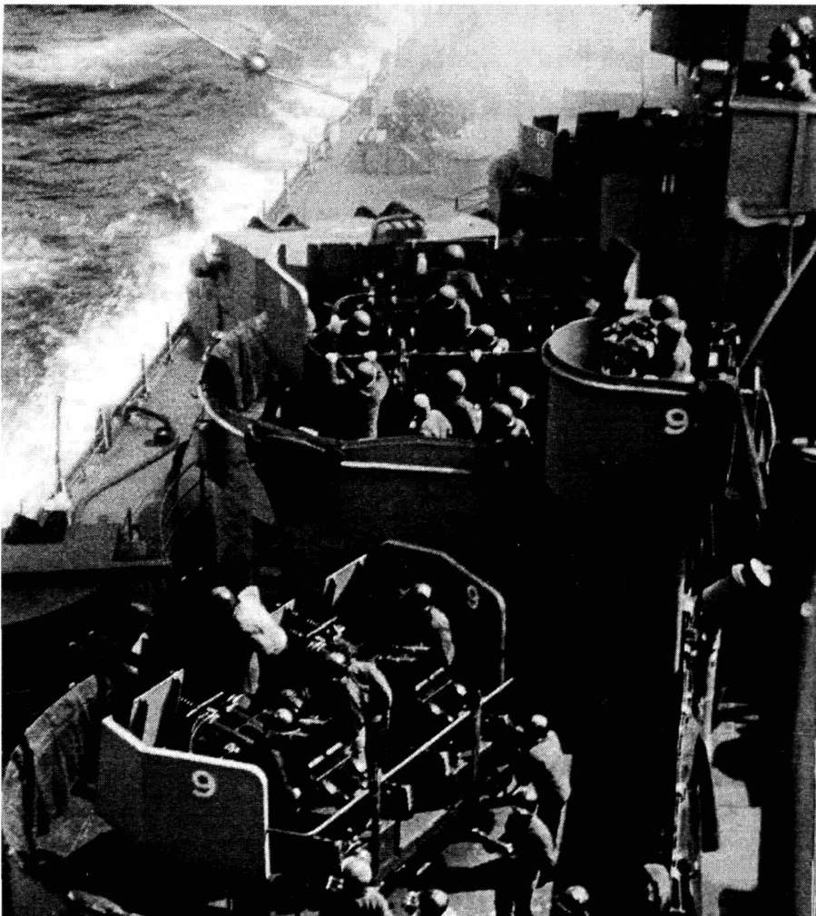
Figure 8-11 (below): While automated fire control fought robot bombs in Europe, remote controls in the pacific faced another novel human/machine combination: Kamikaze attack, here on battleship Missouri . The quad-mounted 40mm gun at lower left (number 9) is under control of the Mark 51 director at center right (also 9). Similarly, the 40mm mount 11 is under control of the director at right (from Edward Steichen ed., US Navy War Photographs (New York: Crown Publishers, 1980), 89).
