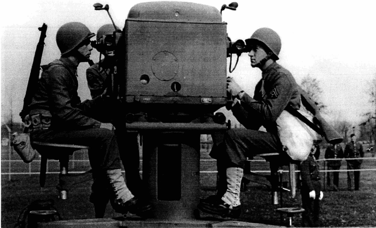
Figure 8-3: M-9 gun director, tracking head with operators. One follows the target in elevation, the other in azimuth. The unit and the operators rotate with azimuth tracking. (AT&T Archives)
