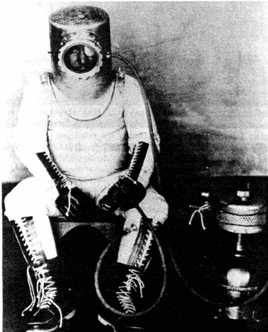
Figure 3-3: Wiley Post in his pressure suit. Note the oxygen tank feeding into the helmet next to Post's eye patch.
