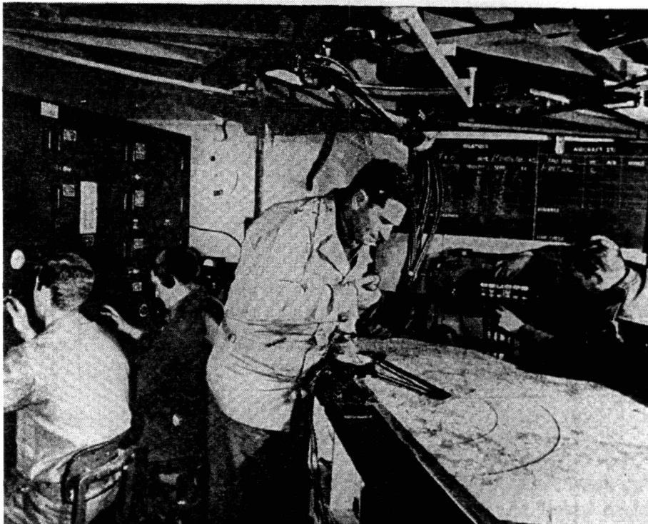
Figure 8-7: Traces on screen and traces of writing, recreating the plotting room in the field. Interior of control van for SCR-584 radar. Note radar operators at left and master plotting board for mapping successive radar tracks. The manual plotting board was later replaced by an automatic, servo-driven plotter built by Bell Labs (Louis Ridenour, Radar System Engineering (New York: McGraw Hill: 1947), 239).
