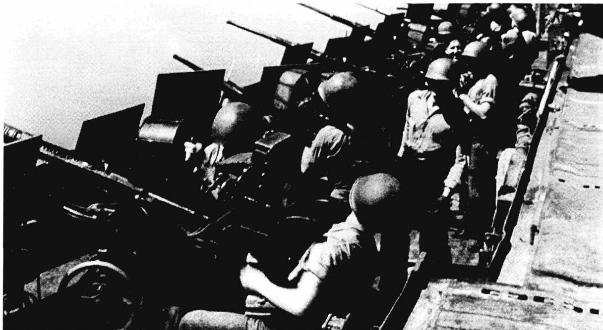
Figure 7-4: Gunners with 20mm Oerlikon guns and Mark 14 sights defending the USS Hornet , February, 1945. (Charles Kerlee, from Christopher Phillips, Steichen at War (New York: Harry Abrams, 1981, 95).
