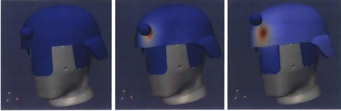
Figure 5-6: Frontal impact simulations are able to model the helmet backface deformation and record the deformation in the clay
