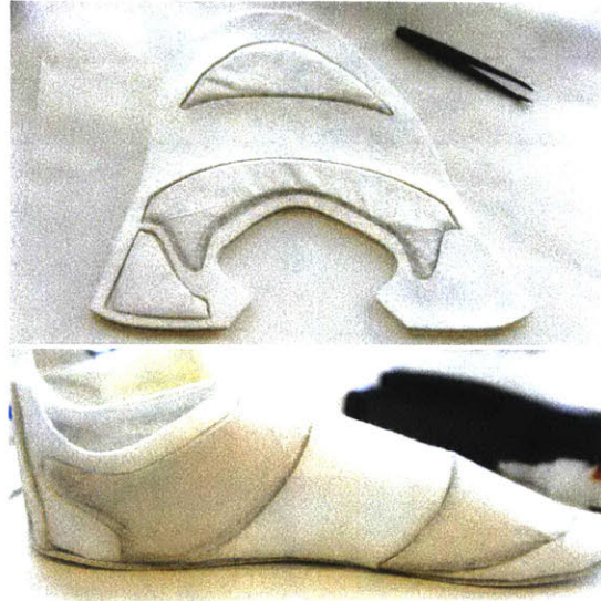
Figure 7.8: One shoe integrates four independently jammable components: the toe box, the heel counter (the part between the heel top and sole) and the upper. For different use scenarios (walking, running, hiking, biking, etc.), different stiffness configurations are possible. Conceptualized by Lining Yao and Jifei Ou. Implemented by Lining Yao.
