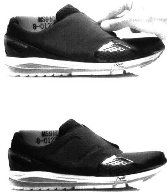
Figure 7.9: We worked with New Balance to fabricate a functional prototype (a stiffness tunable shoe) in its workshop. The shoe is equipped with stiffness-tunable shoelaces, which can automatically tighten up. This functional prototype was co-developed by Lining Yao, Jifei Ou, Daniel Tauber and the New Balance team, led by Katherine Petrecca and Chris Wawrousek.
