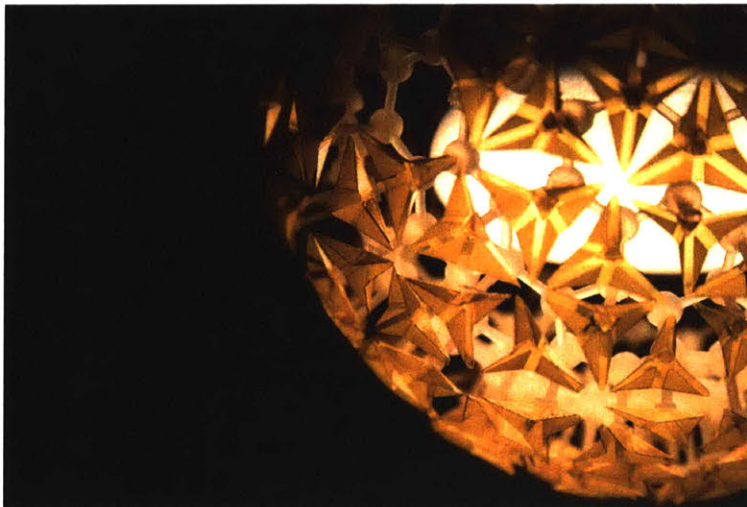
Figure 7.11: Transformable lampshade with tunable lighting permeability. The flaps open up as the temperature rises, causing relative humidity to drop. I prototyped the lampshade together with Chin-Yi Cheng.
