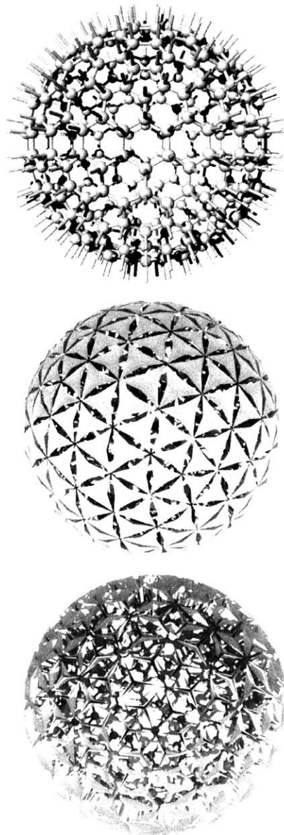
Figure 7.10: The CAD models of the transformable lampshade with tunable lighting permeability. (Top) The scaffold where the transformable units will be patched. (Middle) Transformable units are closed. (Bottom) Transformable units are open. I prototyped the lampshade together with Chin-Yi Cheng.
