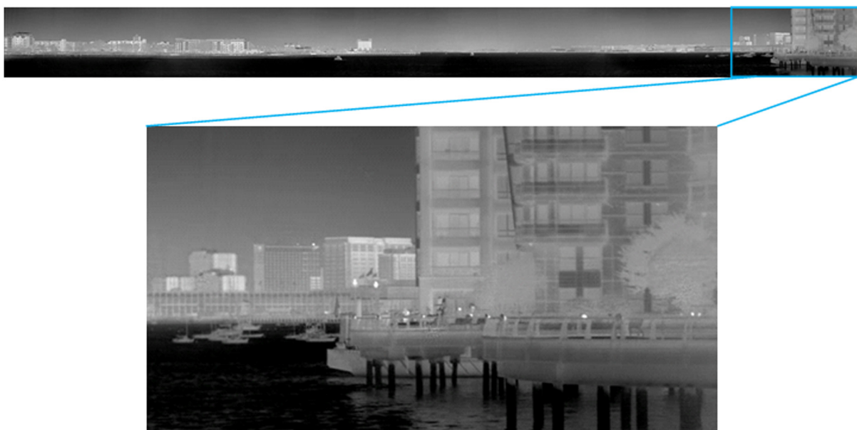
Fig. 15 A single frame from a 90 \times 7.6 deg demultiplexed conventional video. Only the center 1024 \times 512 region of the camera was read out in order to increase the sampling rate.
