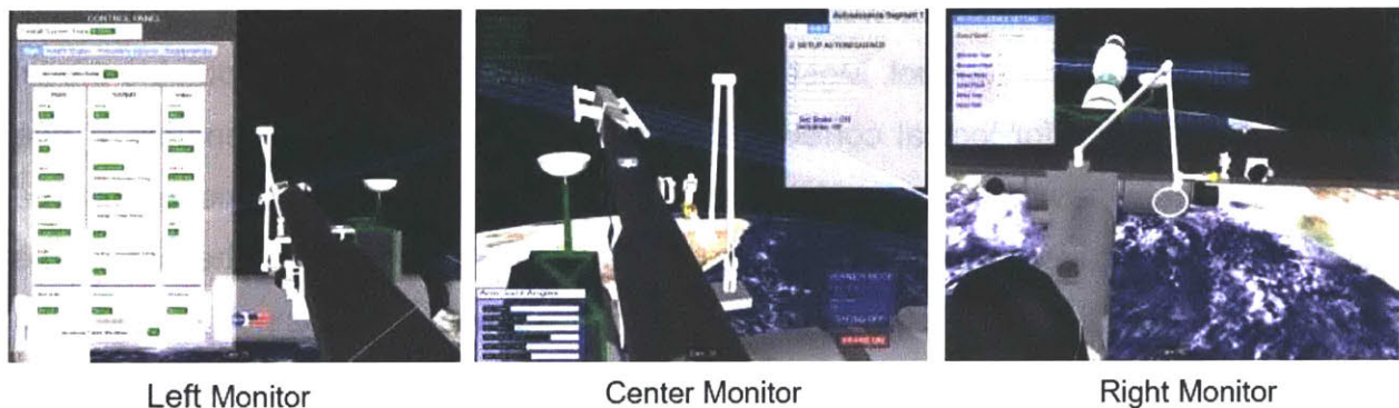
Figure 64: View of Monitors. Left Monitor – Control Panel and “clearance” view, Center Monitor – Electronic Procedure, Joint Angle Display and “task” view, Right Monitor – Autosequence Panel and “big picture” view.
