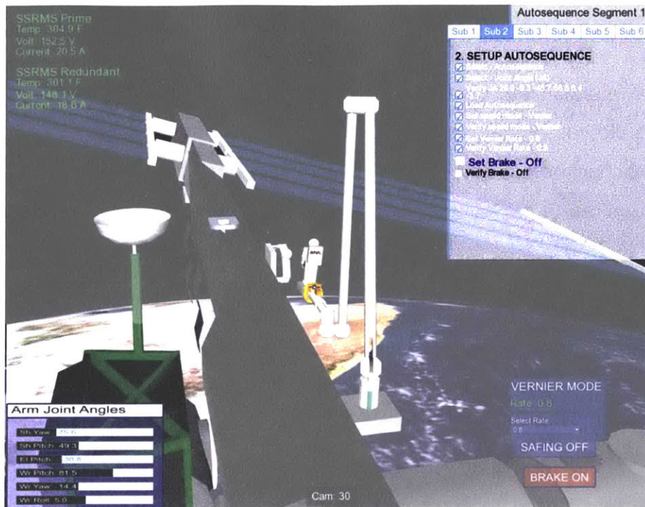
Figure 74: Overview of Center Monitor with Electronic Procedure
