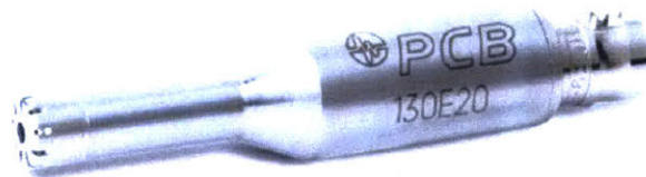
Figure 5-27: Microphone, 130E20 by PCB Piezotronics, to measure acoustic noise emitted from the experimental motor setup.
