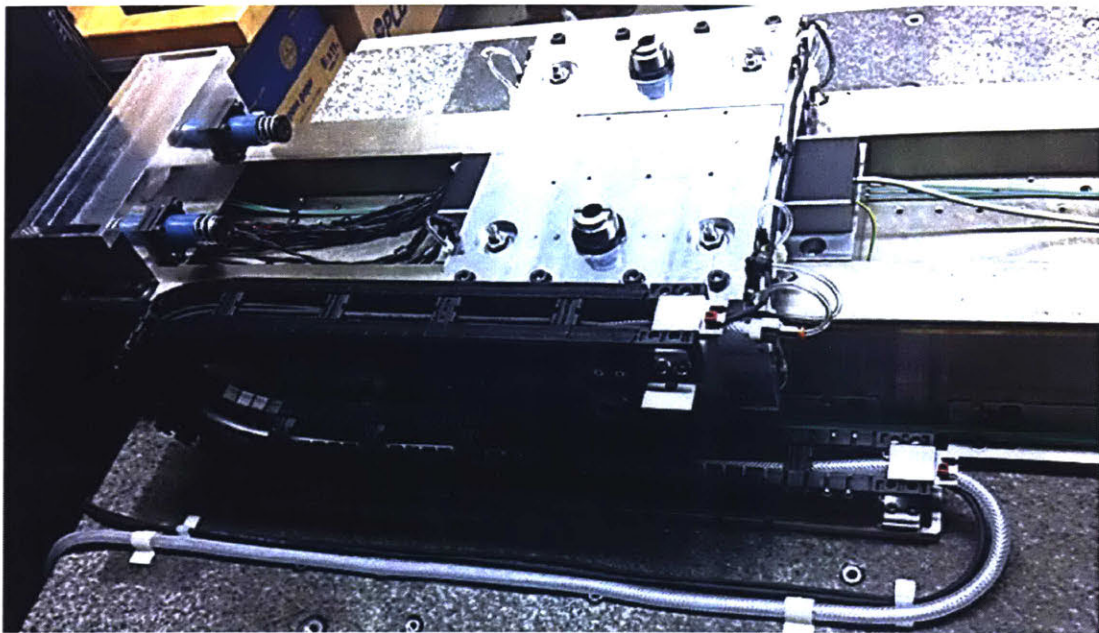
Figure 5-17: Stage testbed with a link-less and hinge-less cable carrier (Quantum 040-28 by Tsubaki) carrying encoder cables and air inlet tubing. Cable stresses are isolated by strain reliefs.
