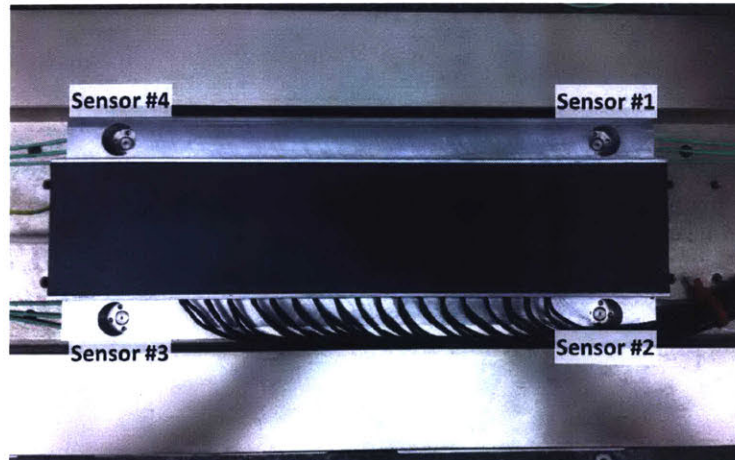
(b) Formed dynamometer with stator mounted on top
