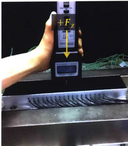
Figure 5-6: Dynamometer Z-direction force measurement test with a force-meter exerting +Z force of 35 to 40 N.
