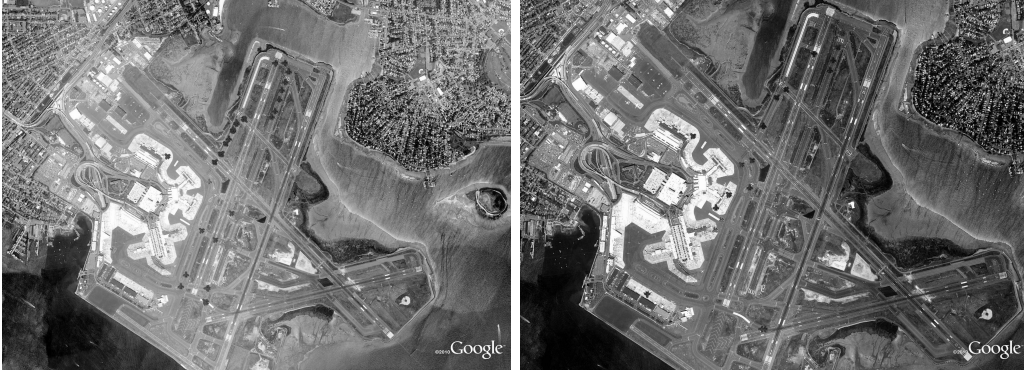
Figure 10: Snapshots of the airport surface, (left) before gate-holds started, and (right) during gate-holding. We note that the line of 15 departures between the ramp area and the departure runway prior to commencement of pushback rate control reduces to 8 departures with gate-holds. The white area on the taxiway near the top of the images indicates the closed portion of taxiway November .
