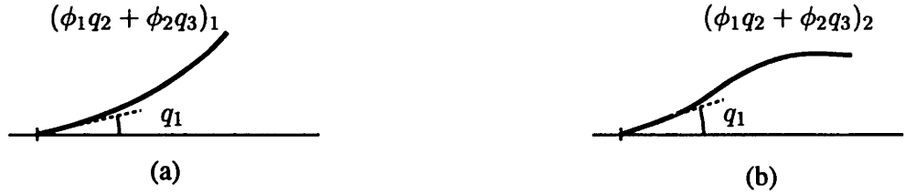
Figure 2-2: Schematic of the ‘Springboard’ mode shapes for; (a) the first coupled mode (in phase) and (b) the second coupled mode (out of phase).
