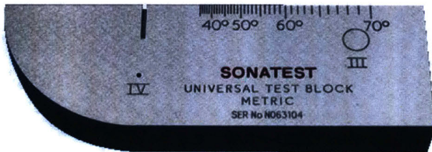
FIGURE 9: CALIBRATION BLOCK USED FOR ULTRASONIC TESTING (SONATEST, N.D)
