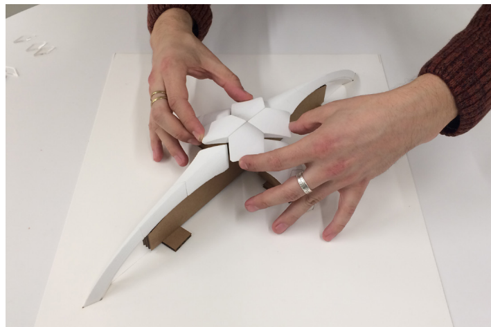
Fig. 3.15. Assembly of scale model on cardboard formwork.
