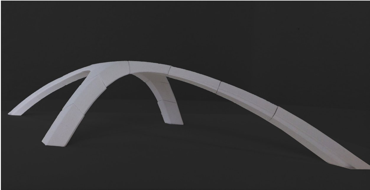
Fig. 3.16. Assembly of scale model. Pieces fit together dry - no glue was used.
