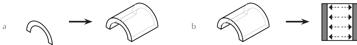
Fig. 3.9. a. Extruding an arch to make a barrel vault; b. Representing a barrel vault in plan.
