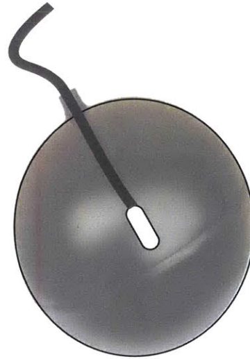
HOB0 Pro v2 Sensor Placed Inside 15.24cm Diameter Black Painted Copper Sphere
