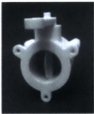
Figure V.5 Throttle valve printed on Dimension SST 1200es with ABS material machine [91]
