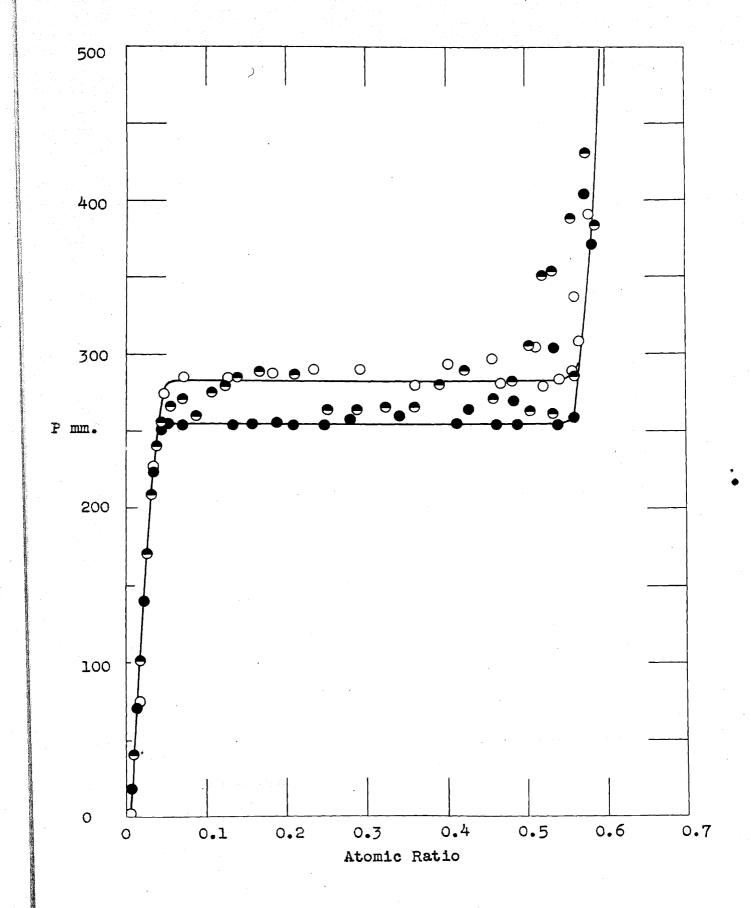
new specimen, Pd 2, agreed quite well with those obtained using a specimen which had been used repeatedly (Pd 1), and which had been in frequent contact with mercury vapor, it was concluded that mercury either had not distilled over to the palladium in appreciable quantity, or had no effect on the hydrogen-palladium equilibrium; so a part of Pd 1 was used again.
