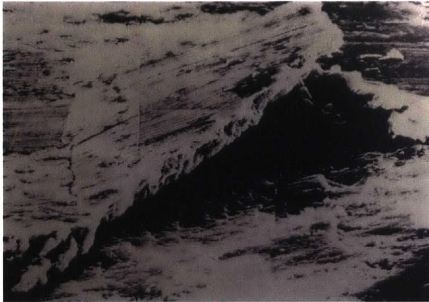
Figure 3.26 An asperity is about to wear off due to fatigue [4]
