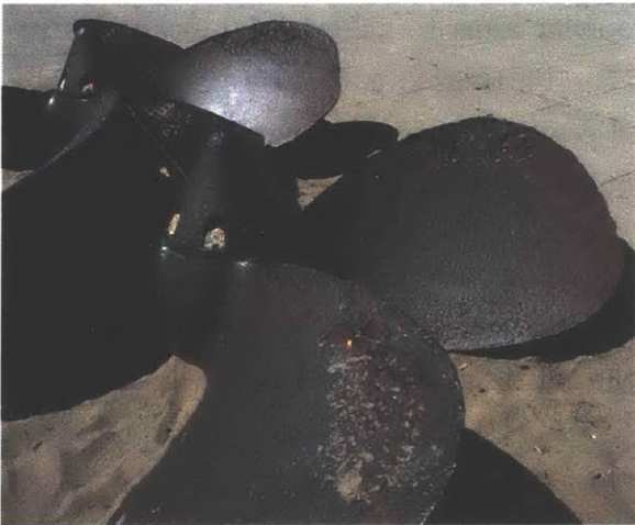
Figure 1-1: The pitfalls of cavitation: propellers showing significant pitting damage [29]
